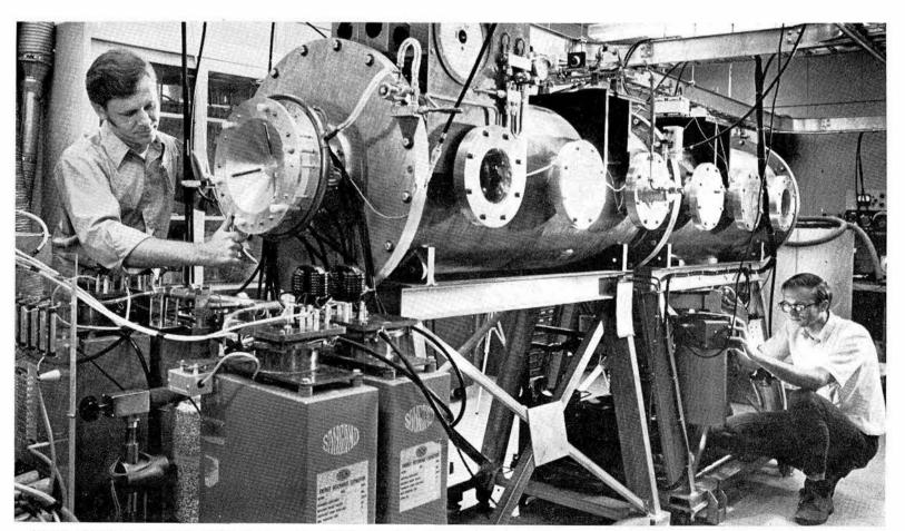
HIGH ENERGY PLASMA GUN designed by Cliff Mendel of Weapons Effects Division 5235, right, has been operating in Bldg. 806 for three months. With Dave Zagar (5235), left, Cliff is striving to accelerate 10<sup>18</sup> argon ions to 3x10<sup>7</sup> centimeters per second. Ion bursts at this speed simulate some aspects of nu-
